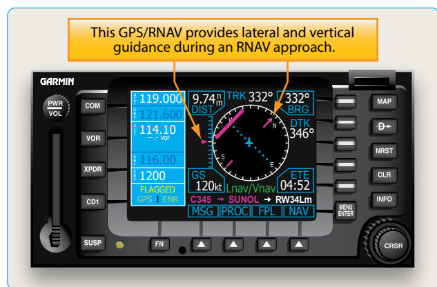
Figure 3-5. WAAS data provide lateral and vertical guidance.
